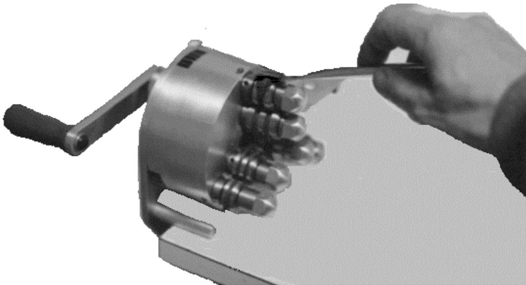
Cleaning the blades consists of pushing the blade guide rings aside so that the supplied cleaning brush can be worked underneath to remove built up lint. Do not bend, twist, or squeeze the blade guide rings as they will not function properly if they are not round.
